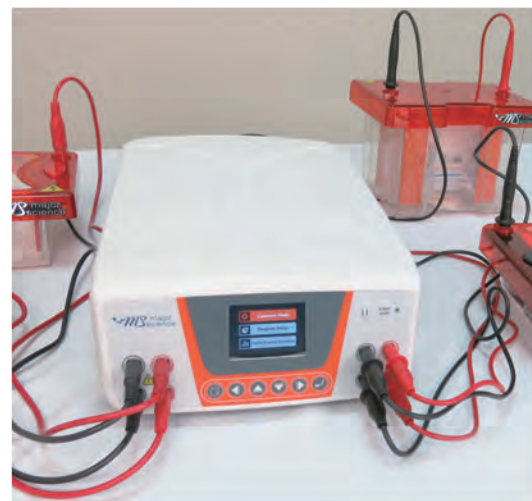
Four pairs of outlet terminals
