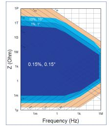
\*High Voltage option module provides up to 10X higher impedance than shown \*Femto ammeter and MREF is used for dielectrics (1 pF to 10 nF) and for high impedance \*Ab obster is used for very low impedance measurements (sub 100 mohm) \*Faraday cage is recommended for dielectric and high impedance measurements
