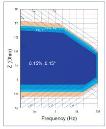
\*High Voltage option module provides up to 10X higher impedance than shown \*MREF is used for dielectrics (1 pF to 10 nF) and high impedance measurements \*Faraday cage is recommended for dielectric and high impedance measurements
