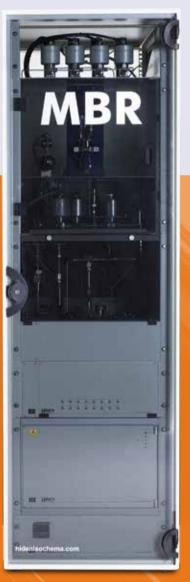
The MBR is a dedicated membrane testing reactor for studying the selective gas permeation properties of membrane materials for separation and purification applications
