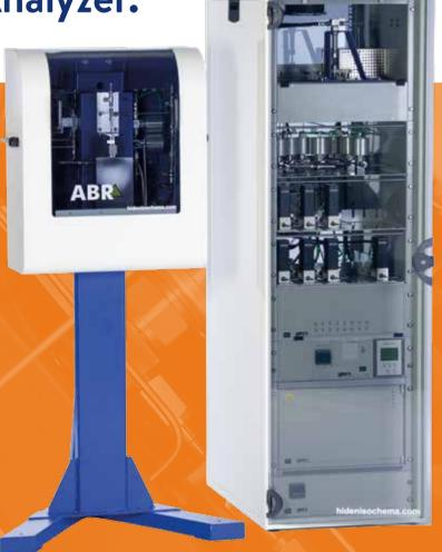
The **ABR** is a dedicated breakthrough analyzer, fully automated and supplied with an integrated close-coupled
