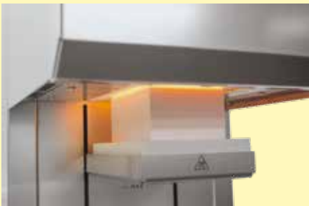
Electrically driven lift-bottom
