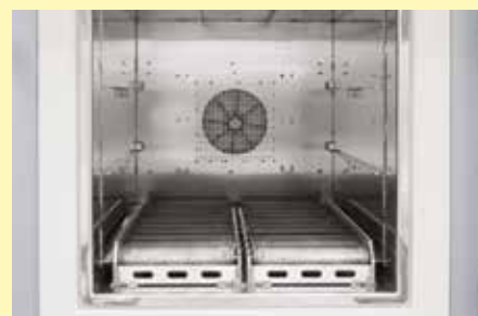
Roller conveyor in furnace chamber
