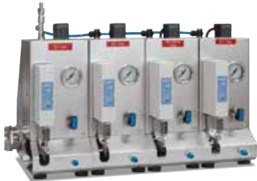
Gas panels with mass flow controllers
