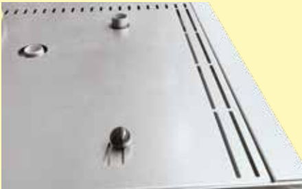
Adjustable exhaust port in the furnace ceiling
