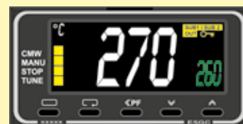
Example of an over-temperature limiter
