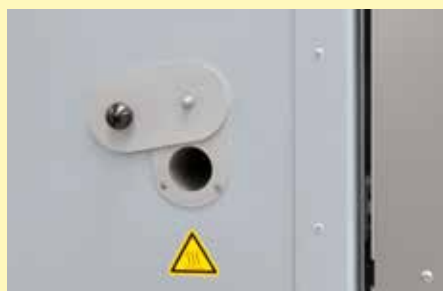
Port for thermocouple
