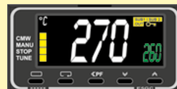
Example of an over-temperature limiter
