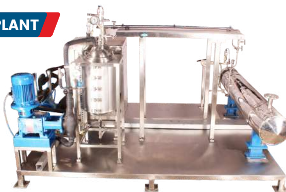
SCCO 2 system for very high temperature (400°C) application
