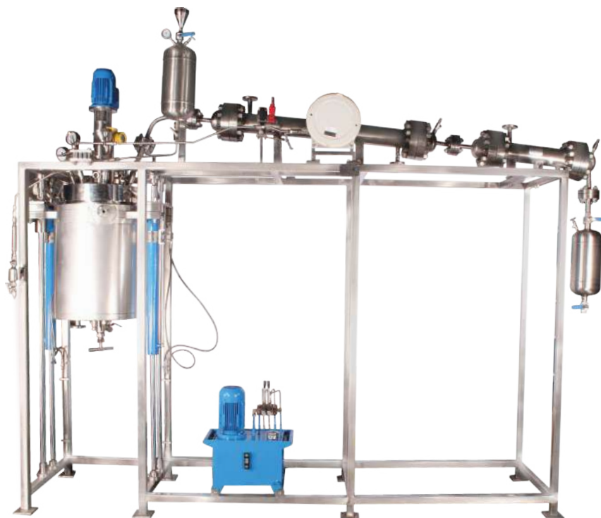
100L reactor with hydraulic lifting arrangement & solvent recovery setup
