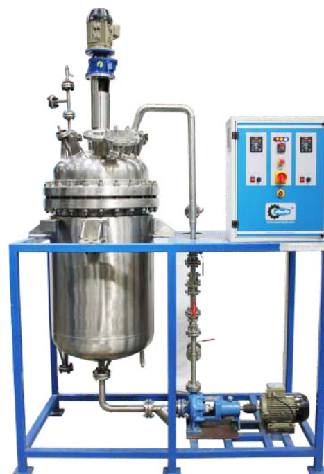
400L Hastelloy reactor with continuous recirculation system
