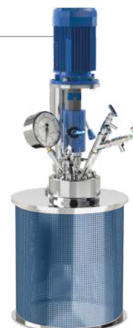
1L autoclave with removable head design
