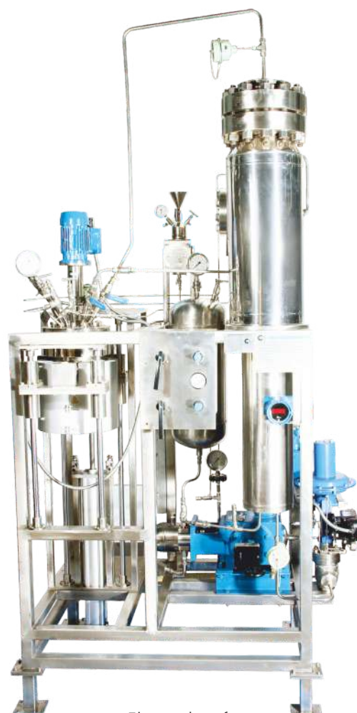
5L autoclave for corrosion testing by weight loss method, electrochemical & recirculation loop
