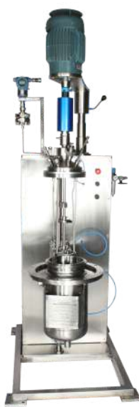
10L with pneumatic vessel raising lowering
