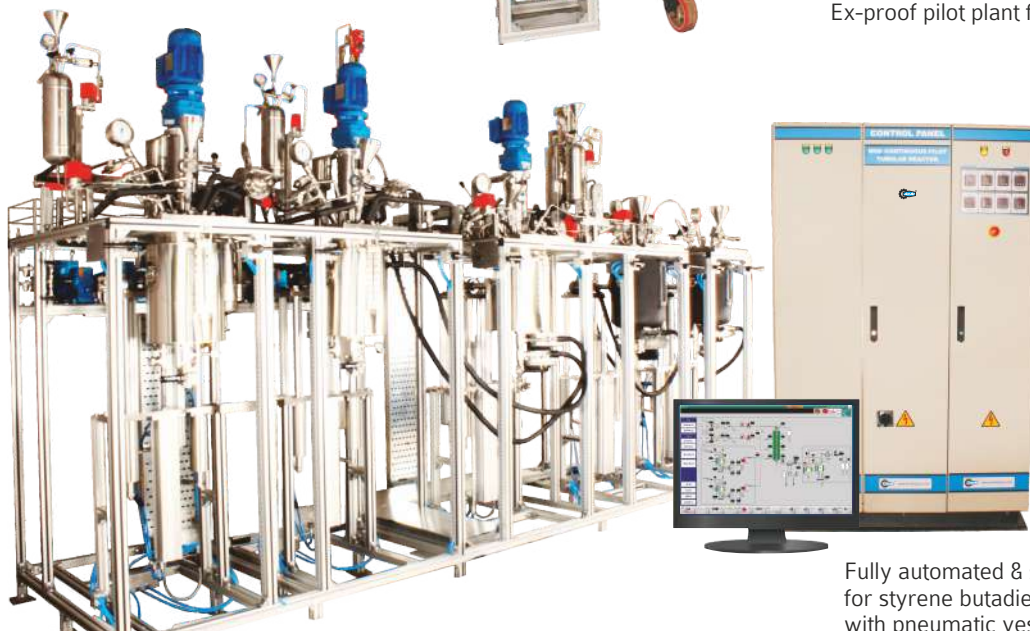
Ex-proof pilot plant for EO-PO reactions
