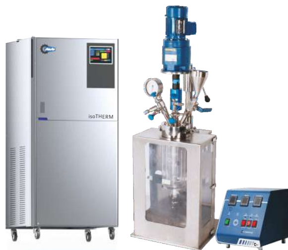
2L Jacketed glass autoclave with temperature control unit
